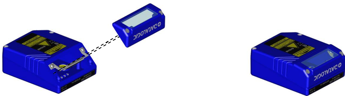
Figure 19 - Mounting a GFC-2020 Deflection Mirror
